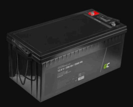
Nominal Voltage: 12.8V **Nominal Capacity:** 200Ah Internal Resistance: ≤220mΩ End of charge Voltage: 14.6V End of charge Current: 100mA End of discharge Voltage: 9.2V Charge Method CC/CV Max Continuous charge current: 100A Max Continuous discharge current: 100A Max Pulse Discharge current: 150A/10S
